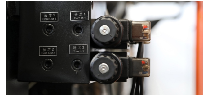
2 sets of core pulls Fulfill product moulding requirements
