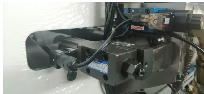
Digital back pressure control Controller-controlled for high precision.
